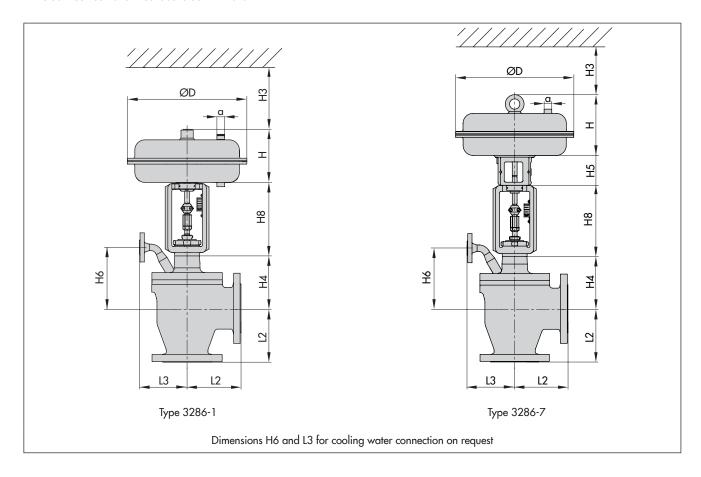
**Table 6:** Dimensions for the standard version of the Type 3286 Steam Conditioning Valve with insulating section
