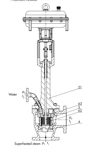
**Fig. 4:** Type 3286 Steam Conditioning Valve with insulating section and Type 3277 Pneumatic Actuator
