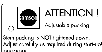
Fig. 3: Label when an adjustable packing is installed
