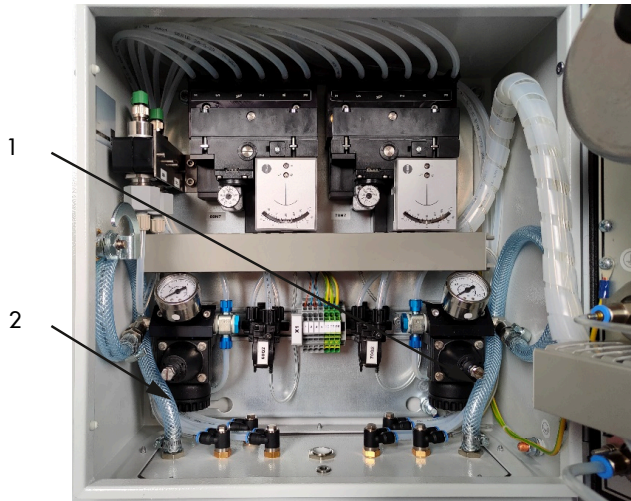
Fig. 16: Setup inside the Type 7311 Air Control System
